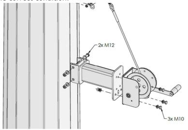
d. It is allowed to mount the hand winch to the adapter first and then mount the prepared set to a dedicated slot on the pole. In this case, remember to check the tightness of the screws securing the hand winch to the adapter.
