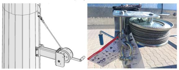
f. Fix the security hand rope (polypropylene braided rope) with a carabiner to the dedicated plate on the pole. This additional hand rope has to be fixed always when the hinge pole is operated down and up. This is safety rope, which is there for the case of any winch mechanism failure. Always 2 persons must operate the hinge poles – one operates a hand winch and one is taking care of the hand safety rope and keeping this one tensioned!
